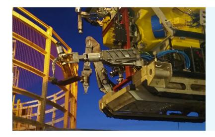
Working in three 12 hour shifts during the 72 hour offshore survey, the Bluefield team completed 37 CPT tests up to 3 m penetration below the seabed. Each CPT test was conducted at 500 m intervals along the trenching route to report on geotechnical conditions of the seabed.
